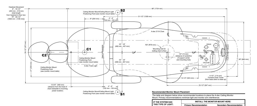
\* If installing at C2, position the monitor mount a minimum of 6-1/2" (165 mm) in front of the track light (towards 12 o'clock).
