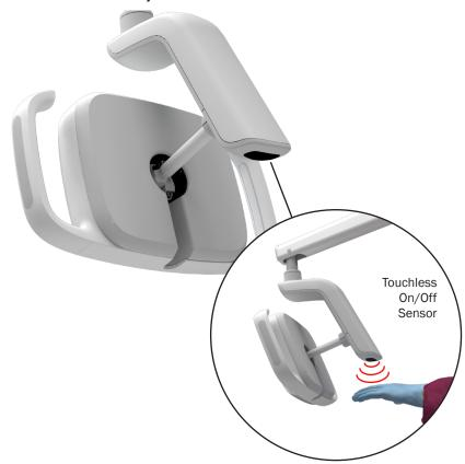
Move your hand within 3" (76 mm) below the touchless on/off sensor to turn the light on or off. If the light does not turn on, verify that the delivery system and/or chair power is on.
