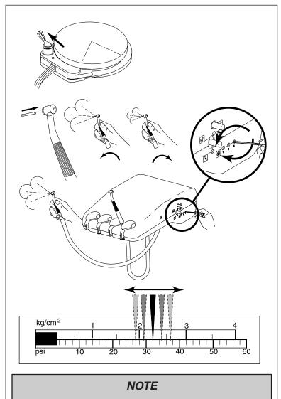
The drive air control must be adjusted to meet the handpiece manufacturer's maximum dynamic drive air pressure specification.
