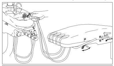
The handpiece tubing flush system flushes more water through the tubings in less time than is normally possible when operating the foot control only. The handpieces should not be connected when flushing the tubings.
