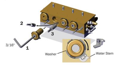
**NOTE** You must turn the retaining washer fully clockwise to secure the water cartridge and retain the stem.
